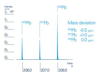
High resolution mass spectra in positive secondary ion mode showing the different Pb isotopes on a silicon wafer.
